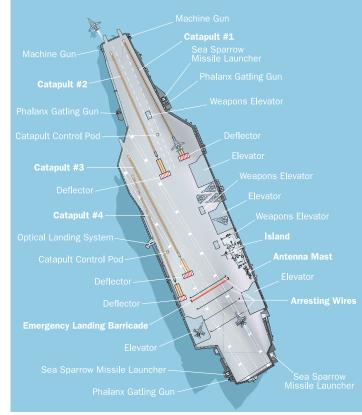
The diagram above shows how these various components fit together. Top View.
